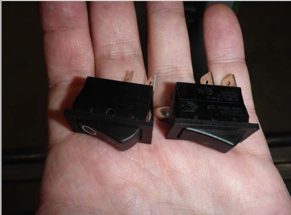
6. With the new switch mounted securely, place the wires located on the inside of the control box onto the new switches prongs.
