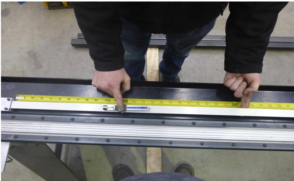
**Take your reading from the left most side of the blue plastic gauge arm where it meets the number scale on the gauge.**
