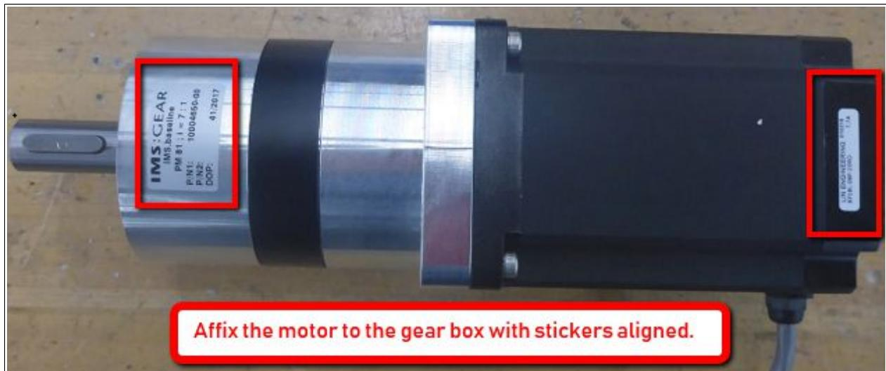
10. With the stickers facing UPWARD, return the assembly to the motor mounting plate on the chuck trolley. Affix with the 5mm bolts (x4).
